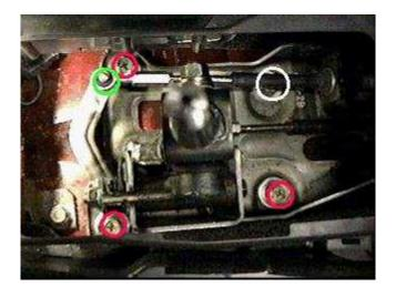
You'll see 4 bolts on the bottom of the shifter base. One will be blocked by a shifter linkage [white circle]. Remove the cotter pin from that cable [green circle]. (You bend the two ends back to straight again and pull it out of the hole) Remove the four bolts. You can use a Phillips to unscrew the bolts once they are loosened. If you can reach/access the bolts with your socket extension and normal size socket then skip the next paragraph. The other red circles show the remaining bolts.
