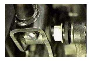
Reassemble the shifter mechanism. Remember the smaller ends of the two nylon bushings face each other. Be careful when tightening the 14mm nut - make sure both bushings are in place, you don't want to crush one of them.
