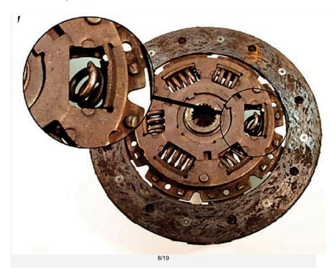
Clutch Disc Hub Springs Loose/Missing Symptoms:
